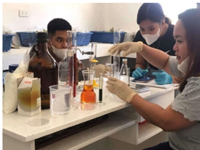
Fig. 6: Vitamin C Titration. The titration was performed using iodine solution in buret. The final amount of titrant used on the standard vit. C and lettuce samples were titrated to blue black color end point to calculate the vitamin C content of lettuce.
