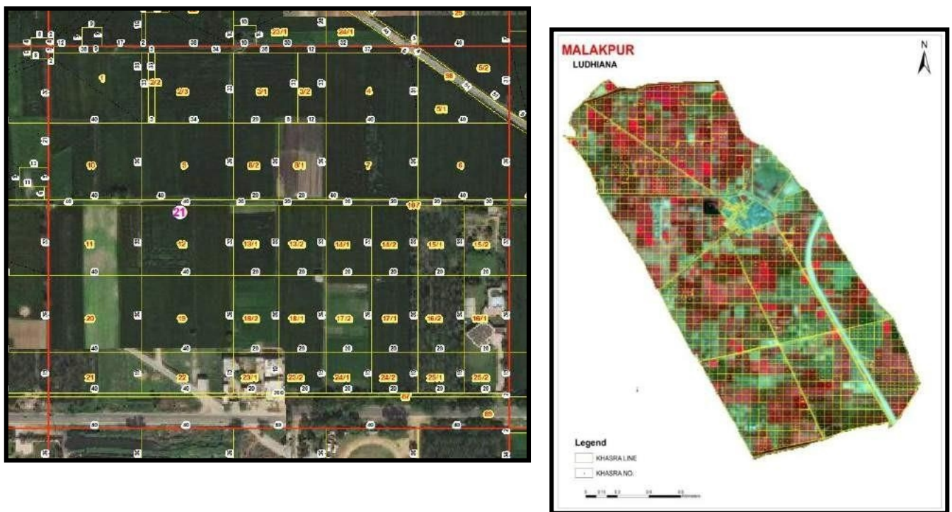
Figure 5: (a) Georeferenced Cadastral Map and (b) Enhanced section of the Georeferenced Cadastral Map.
